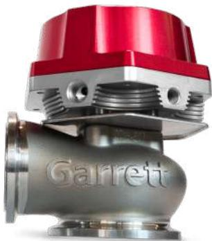
**G**arrett Vent | External Wastegates regulate turbocharger shaft speed by venting exhaust gas around the turbine stage of the turbocharger. CFD optimized design maximizes flow and delivers optimum boost control. Advanced thermal optimization increases durability of the diaphragm. The cap design makes spring changes and serviceability of the entire GVW lineup easier and more reliable to perform.
